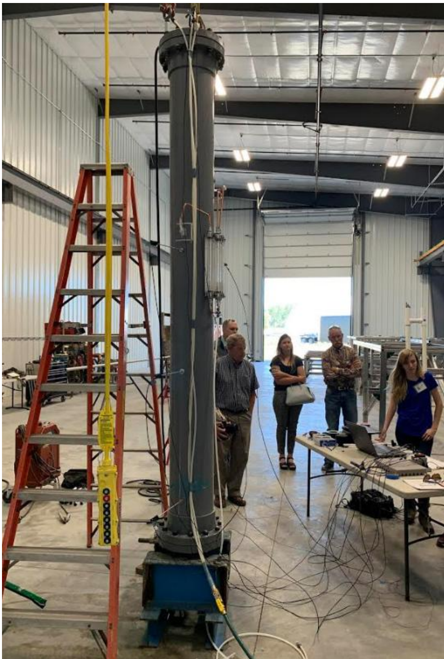
University of Idaho faculty and students and Premier Technology staff run the Molten Salt Nuclear Battery testing device for the first time, using ohmic heating to evenly heat the reactor's liquid fuel via an electric current.
