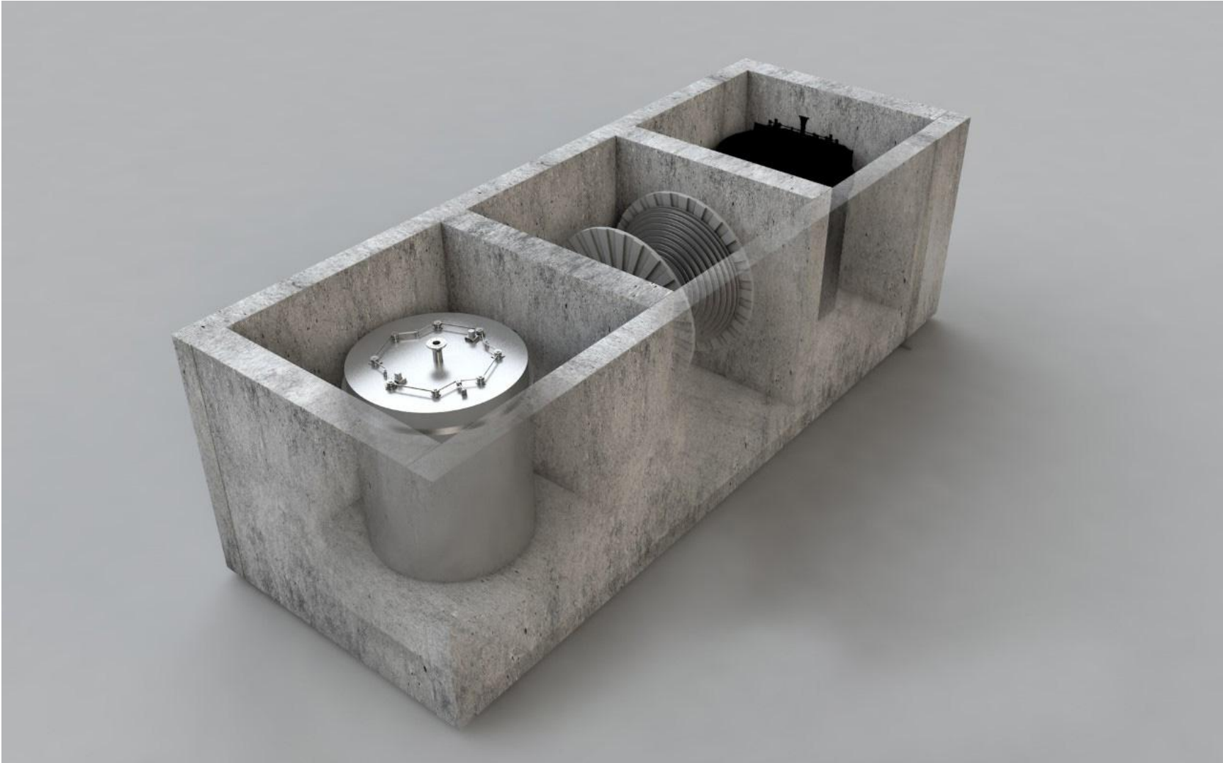
Artist's rendering of University of Idaho Molten Salt Nuclear Battery reactor design next to power conversion unit.
